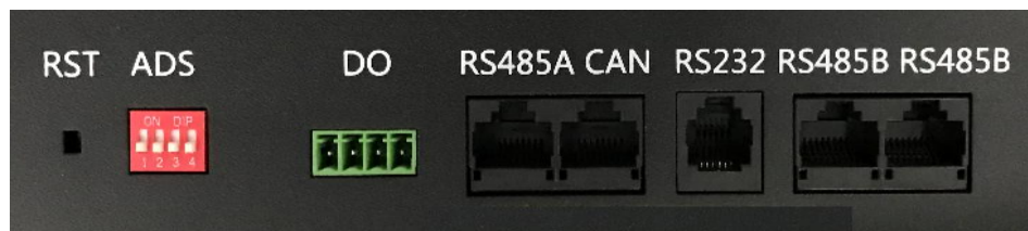
Figure 15. this is 4bits coder and communication port.CAN port and RS485A port can be selected as the same time.
